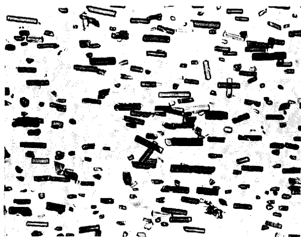
Fig. 4.1. Microcrystals (10–100 \mu\text{m} ) of the protein met-aquo-myoglobin suspended in aqueous ammonium sulphate solution are almost completely oriented by a homogeneous magnetic field of only 0.3 T applied for 5 min. The protein carries a high-spin iron in the planar porphyrin group which is responsible for substantial anisotropy of the paramagnetic susceptibility due to some spin-orbit coupling even at room temperature. The observed magnetic orientation is very probably of paramagnetic origin because microcrystals of diamagnetic CO myoglobin do not orient even in 8.5 T [4.57, 58]
