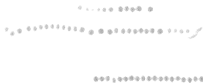
Fig. 4. Chains formed by the magnetic particles in a magnetic field of 125 mT.
