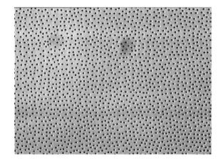
FIG. 1. A typical image  $(500 \times 380 \ \mu\text{m})$  of our two-dimensional colloidal model system with paramagnetic colloids of  $d=4.7 \ \mu\text{m}$  diameter. The particles interact via a potential  $\sim \Gamma/r^3$  in which the interaction strength  $\Gamma$  can be conveniently varied through the external magnetic field.
