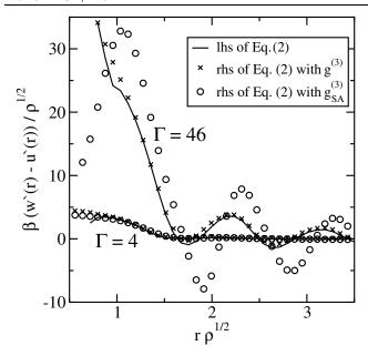
FIG. 5. Test of Kirkwood's approximation using experimentally determined three-particle distribution functions ( $\Gamma=46$  and  $\Gamma=4$ ). Solid lines for the left-hand side of the Born-Green equation [Eq. (2)], symbols for the right-hand side, evaluated using the full triplet distribution function  $g^{(3)}$  (crosses), and the distribution function  $g^{(3)}_{SA}$  (open circles) which is based on Kirkwood's superposition approximation.
