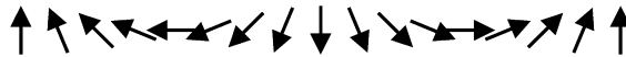
Fig. 2.1 One-dimensional wave of magnetic moments with lowest wavelength. The orientation angle of the moments varies in the range [0, 2\pi] over the system size L .
