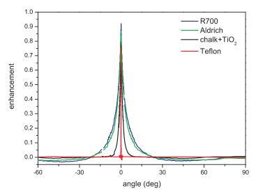
Fig. 2: (Colour on-line) Measurements of backscattering cones for different samples. As the cone width increases, more energy needs to be compensated. Thus the most turbid samples (R700 and Aldrich) lead to a noticeable energy cutback at angles around 45°. The amplitude of this cutback is reduced with decreasing turbidity, but stays positioned around 45°. This indicates that the cutback is due to effects occurring at a fixed length scale close to  $\lambda$ .
