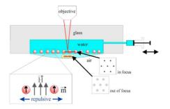
With superparamagnetic colloids at the air water interface we are able to realize a quasi ideal 2D colloidal system (less than  $1\mu m$  Deviation from perfect flatness of the surface). This system is very powerfull to modelise large variety of situations concerning hot physics topics.
